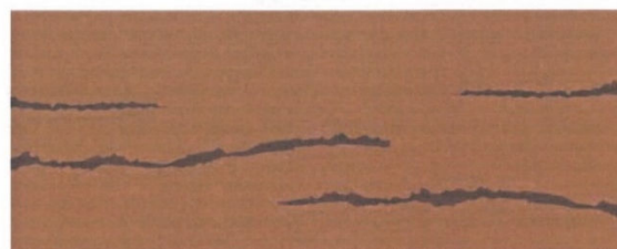
Figure 7. Natural pans – often very hard bands of soil particles cemented together by iron and manganese
