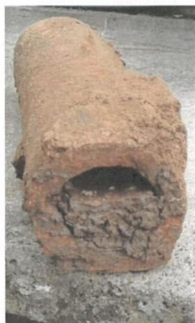
Figure 22. Silted clay drain
