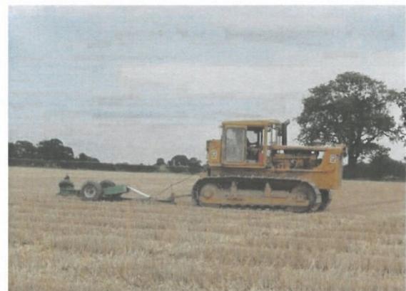
Figure 30. Installing mole drains
