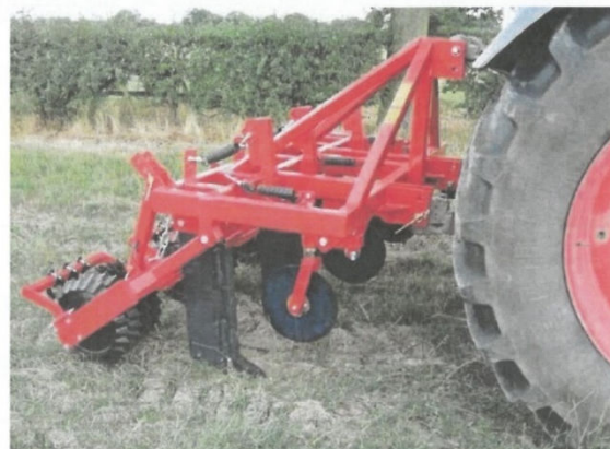
Figure 11. Topsoil loosener for grassland
